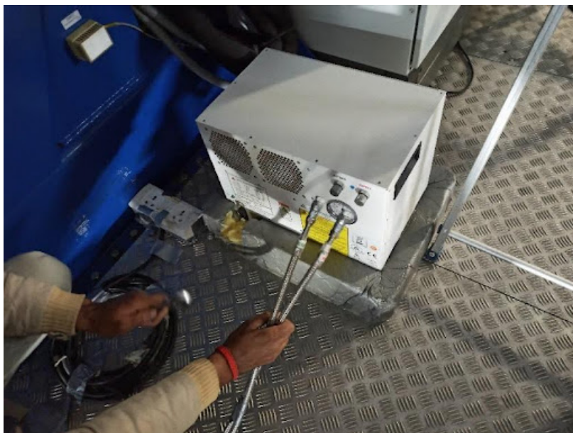
Figure 14: The compressor used for cooling the CCD
