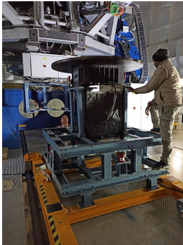
Figure 5: The ADFOSC being carried below the telescope.
