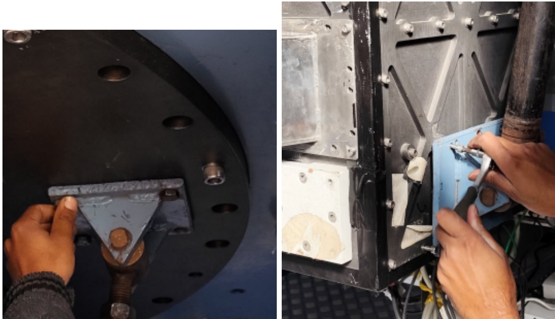
Figure 11: The flexure rods of ADFOSC.
