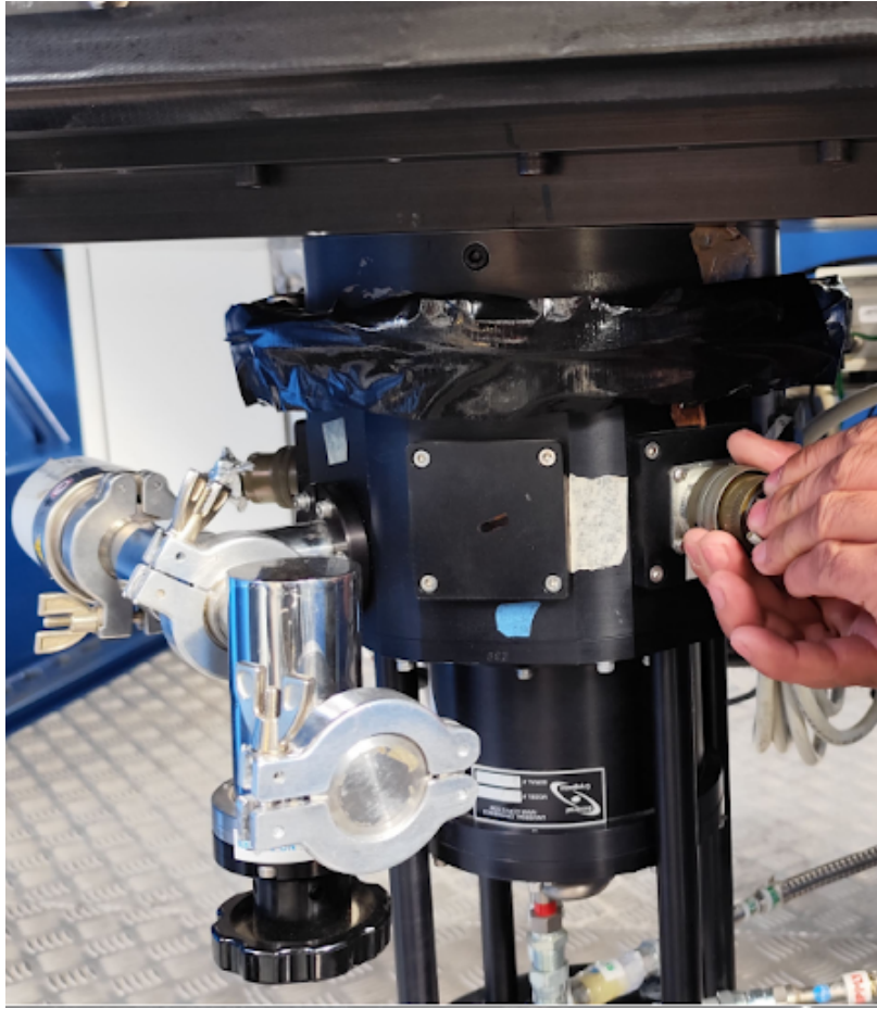
Figure 13: The mounting position of the CCD below the instrument.
