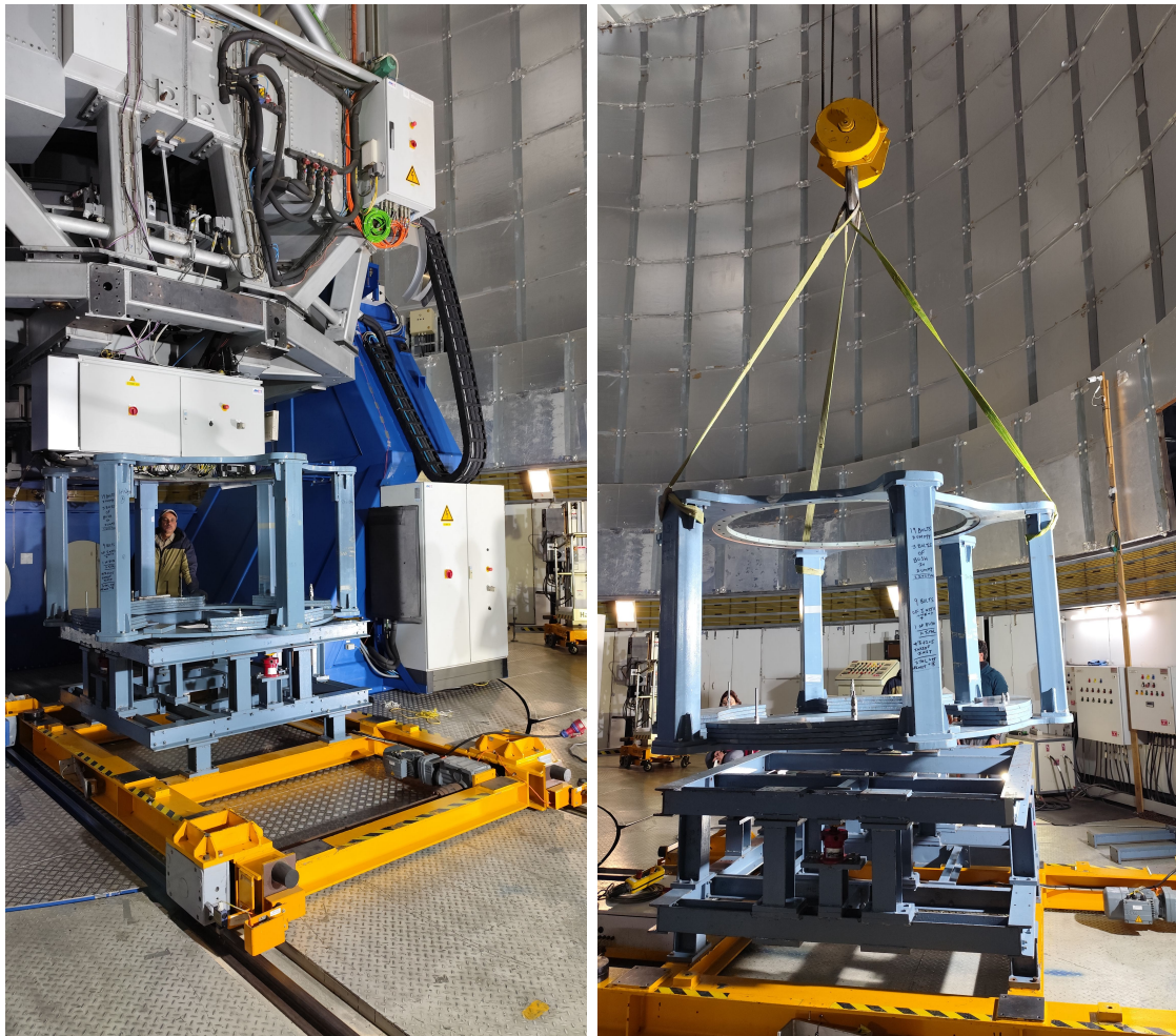
Figure 24: Top to bottom: Move the dummy with the help of the transfer trolley then transfer it to the ground floor.
