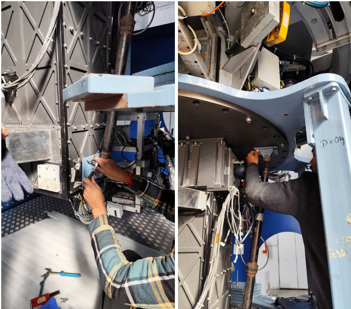
Figure 13: Remove the flexure rods by unscrewing them from the bottom and top.
