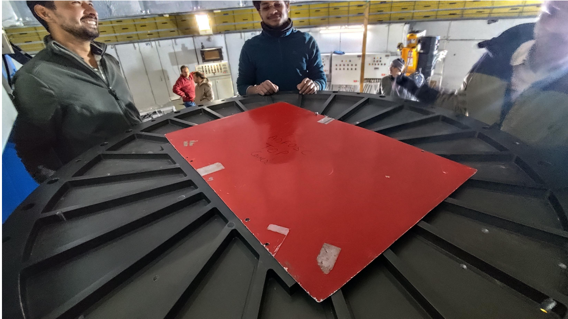
Figure 19: Cover the ADFOSC with the designated red colored plate.
