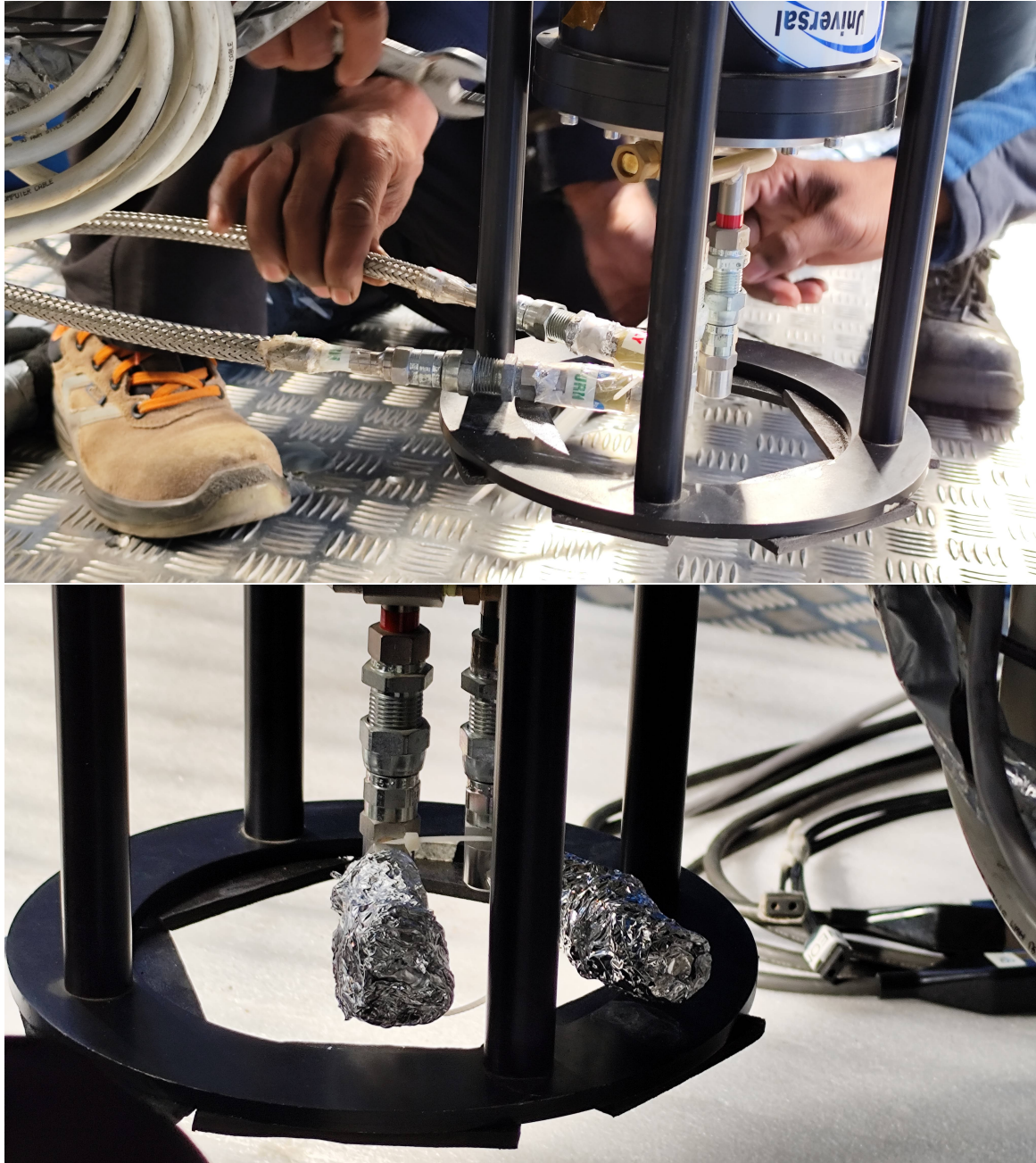
Figure 4: Top to bottom: Removing the coolant supply and return wires connected to the CCD. The ports should be covered with aluminum foil as shown in the figure.
