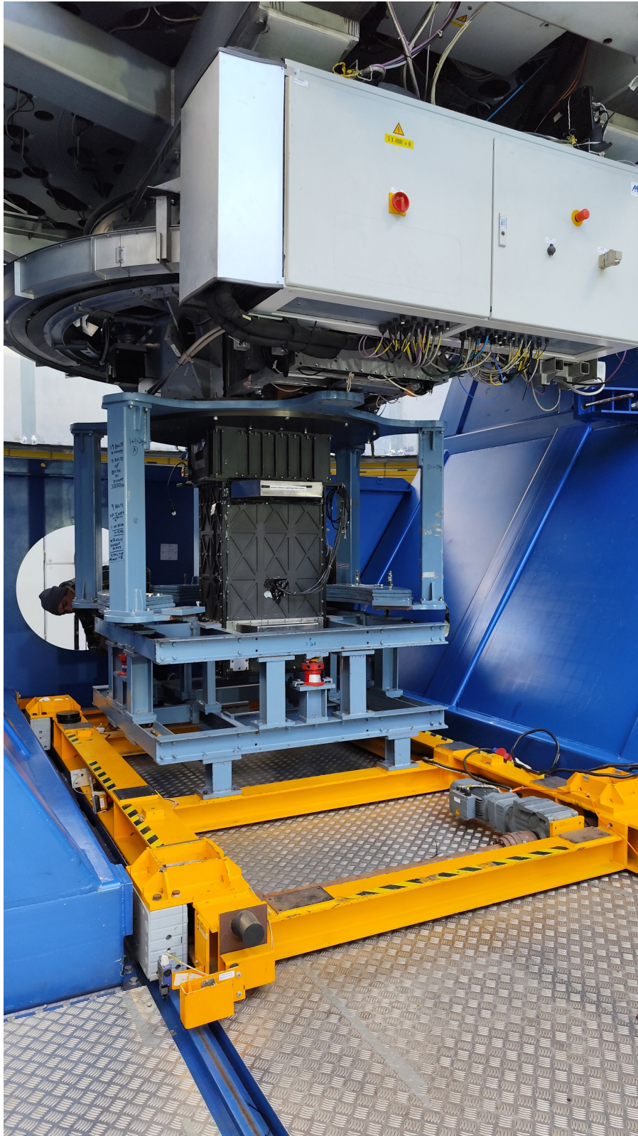
Figure 14: Move the transfer trolley below the instrument.
