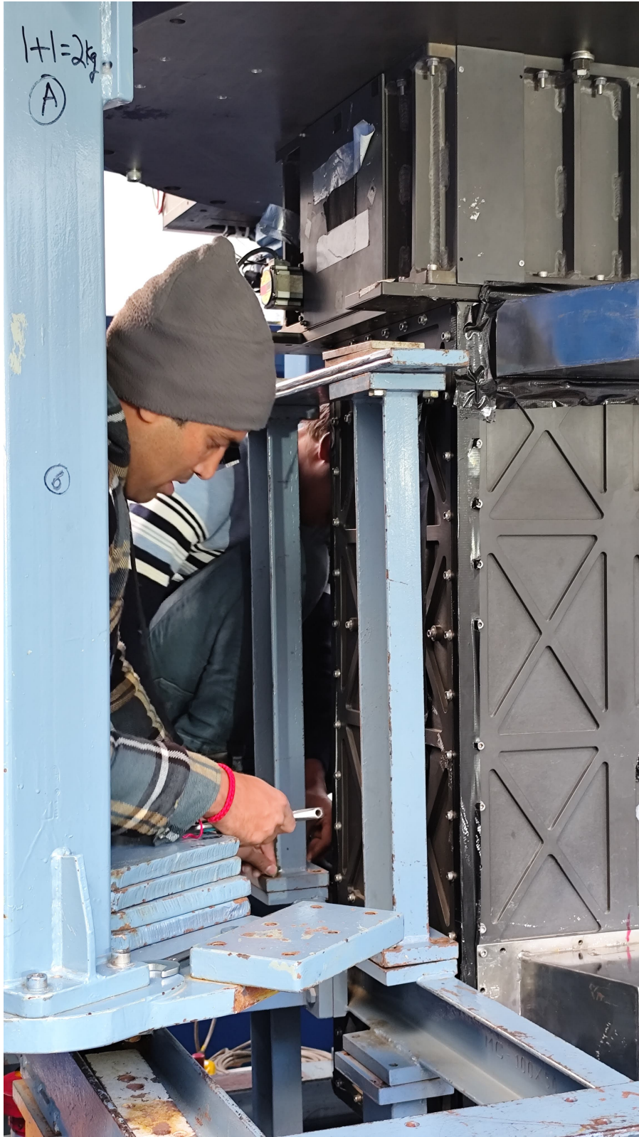
Figure 15: Mount the stands on both sides of the instrument.
