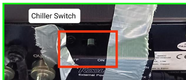
**Figure 12:** The chiller can be turned on by the black switch indicated by the red box.
