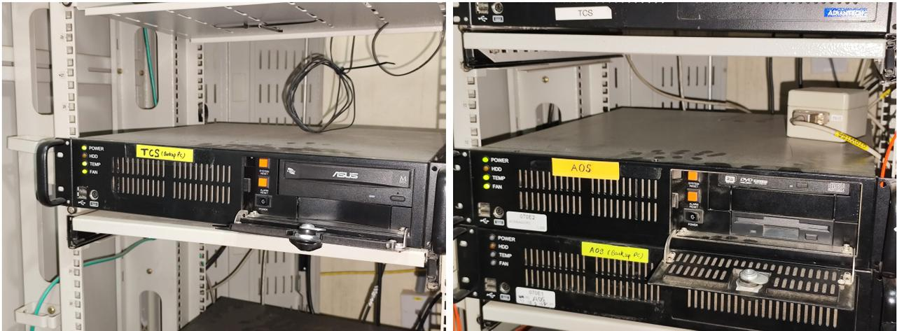
Figure 4: The TCS and AOS PCs in the cabinet of the control room.
