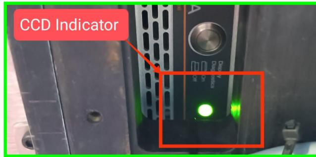
**Figure 13:** The CCD can be turned on using the push button.
