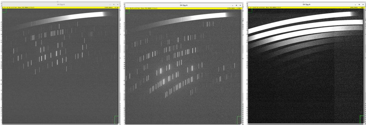
**Figure 13:** The calibration lamps obtained from TANPEC are shown in the figure. Left panel shows Argon, middle panel shows Neon, and right panel shows Continuum.
