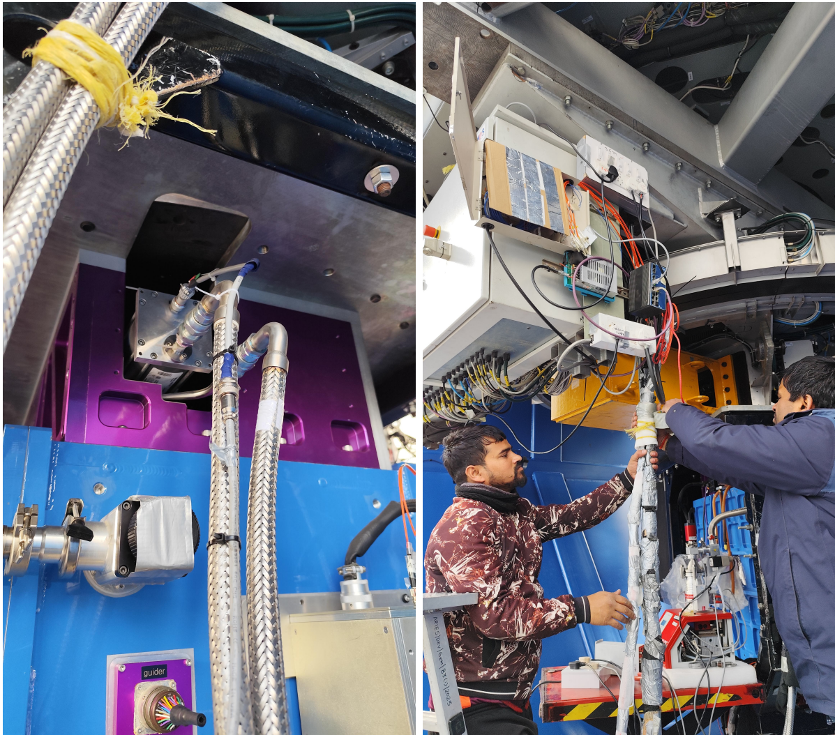
Figure 10: Connect the coolant pipes to the instrument and secure them with the vertical pipe.
