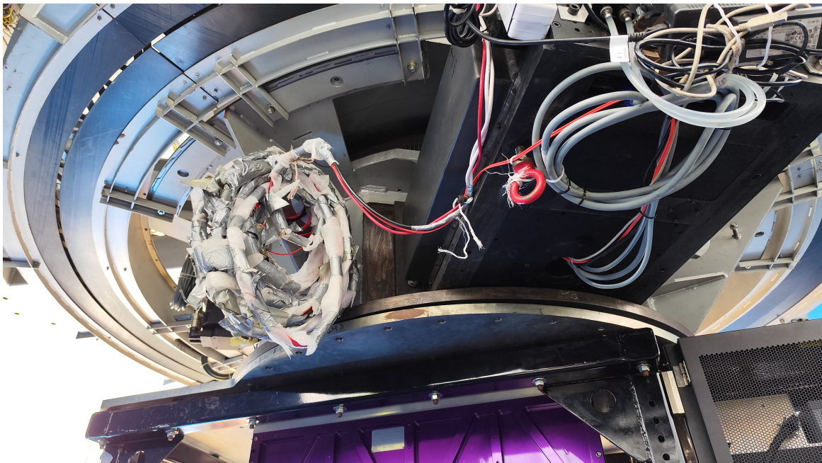
Figure 7: Secure the wires of side port instruments.
