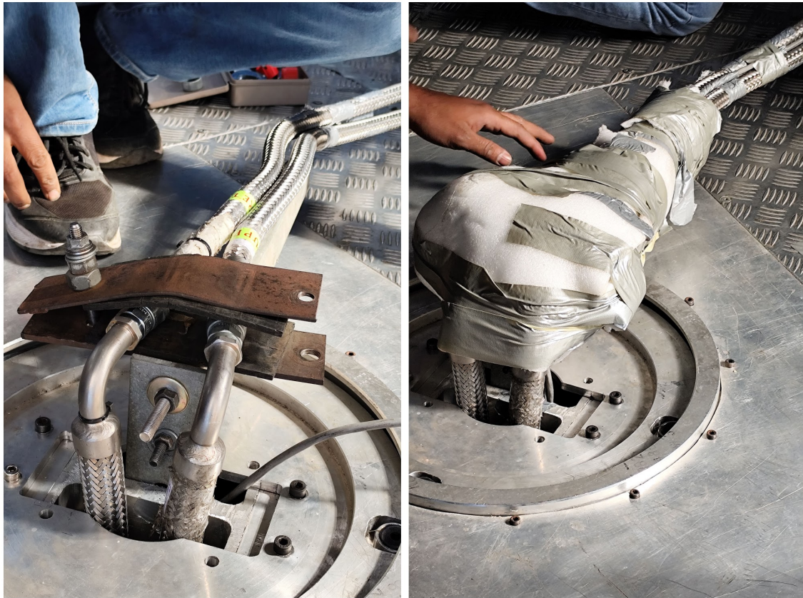
Figure 9: Secure the coolant pipes with a clamp and thermocol paper.
