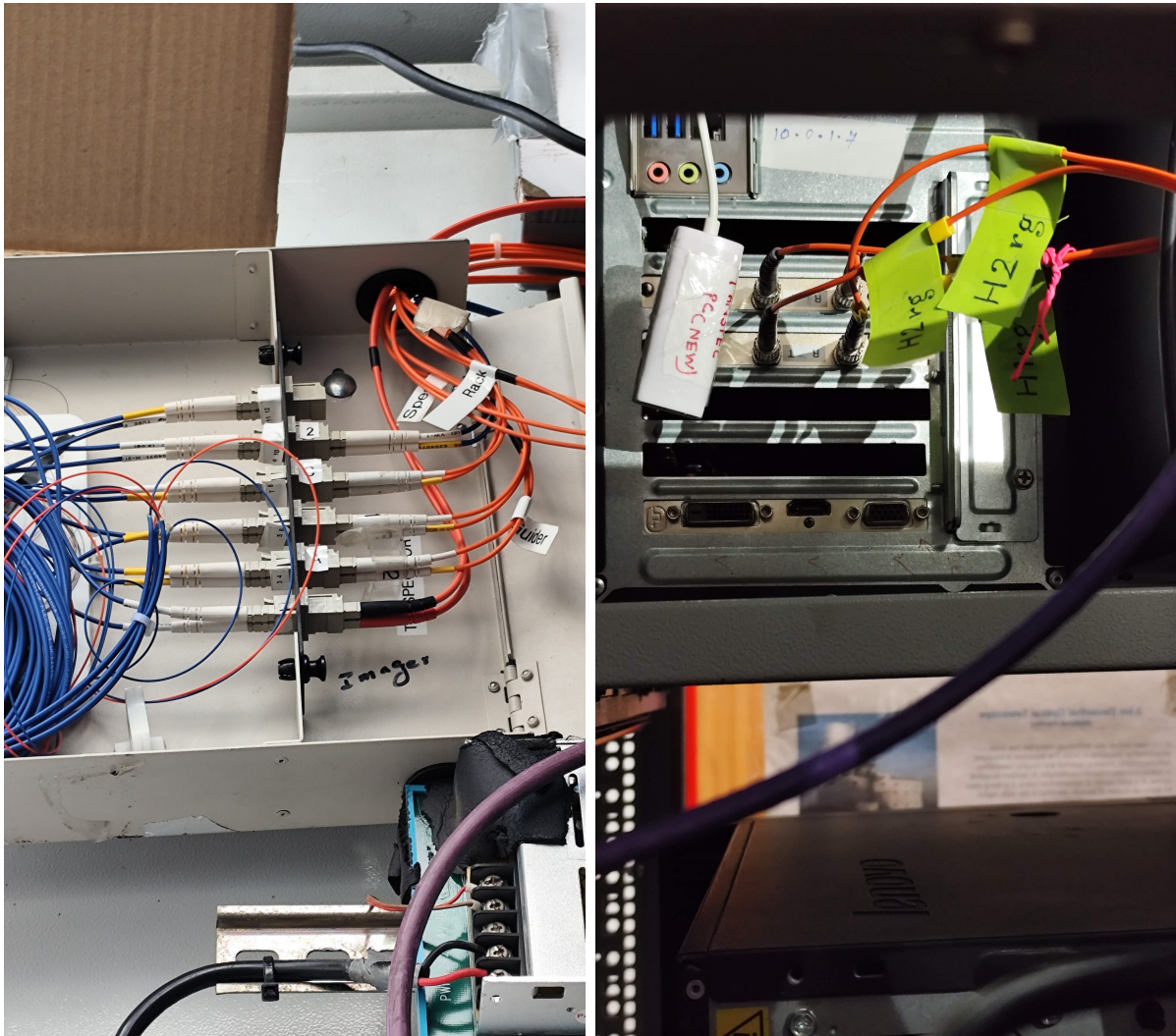
Figure 12: Connect the optical fibers to the distribution box located on the telescope and TANSPEC PC.
