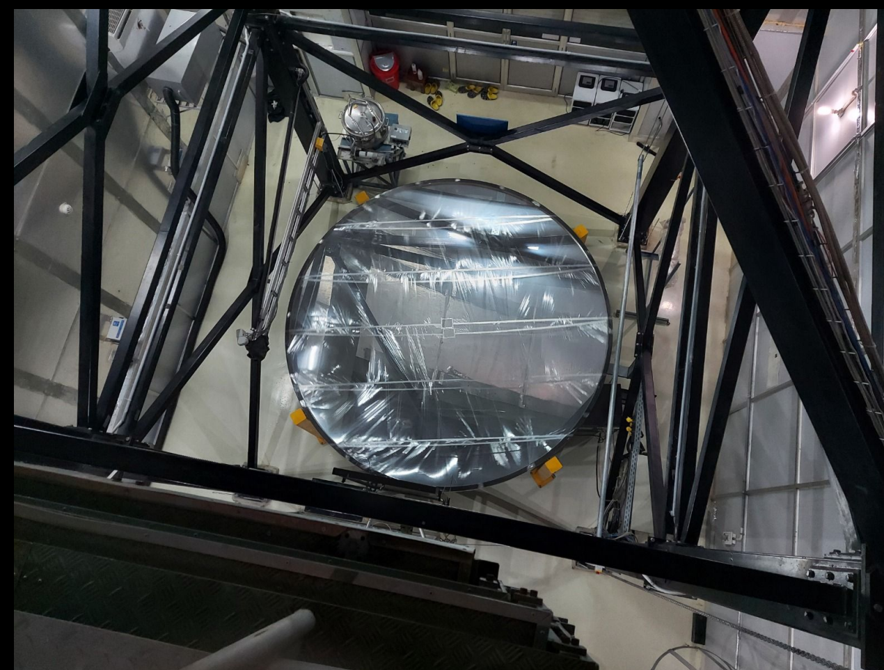
Top view of the liquid mercury mirror covered with a mylar sheet.
