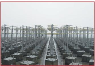
Installed profiler (49 subarray) at ARIES, Nainital
