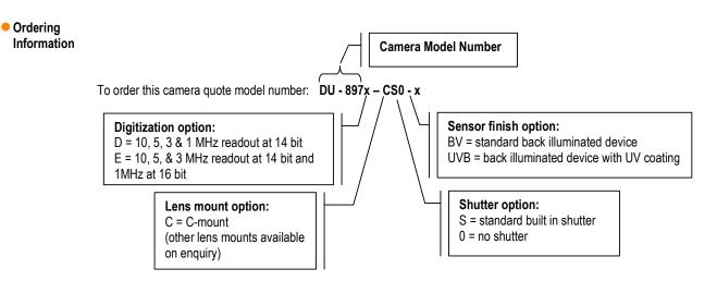
e.g. DU-897D-CS-UVB is a back illuminated iXon EM + DU-897 camera with 14-bit digitization at 10, 5, 3 and 1MHz readout speeds, EMCCD and conventional output amplifiers, standard shutter and UV-enhanced coating.
