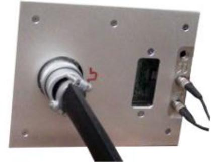
Leach controller Power cable and optic fiber
