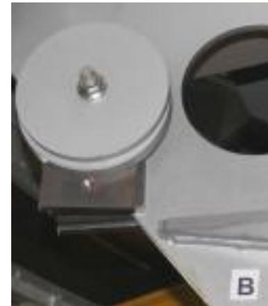
Dummy weight on triangular plate B
