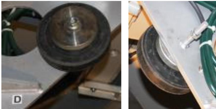
Dummy weight on triangular plate D
