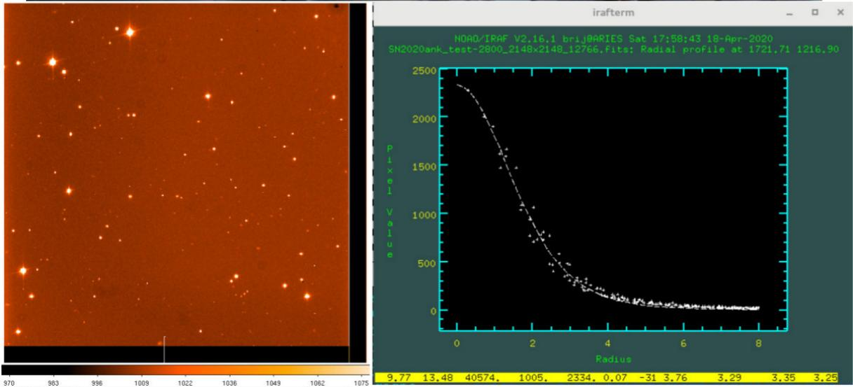
Figure 3.4: Top: The picture of IMAGER instrument mounted on the main-port of the telescope. Bottom-left: A 30s R-band image of a  $6'.5 \times 6'.5$  field centered at SLSN 2020ank taken on 16th March 2020 using IMAGER with pixel binning of  $2 \times 2$ . Bottom Right: Image profile of a stellar source of the same field. The PSF FWHM is 3.25 pixel ( $0'.62$ ).
