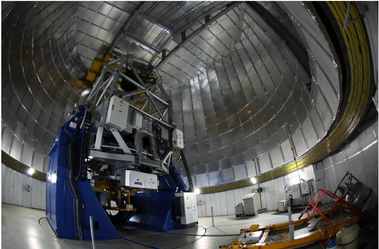
Figure 3.1: The fish-eye view of 3.6m telescope inside the rotating dome structure - courtesy Anna
