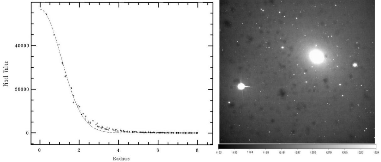
Figure 3.5: A view of the ADFOSC mounted on the main-port of telescope. Bottom-right: A 30s r-band image of a  $13'.6 \times 13'.6$  field centered at SN 2020ue taken on 27th May 2020 using ADFOSC with pixel binning of  $2 \times 2$ . Bottom Left: Image profile of a stellar source of the same field. The PSF FWHM is 2.3 pixel ( $0''.92$ ).
