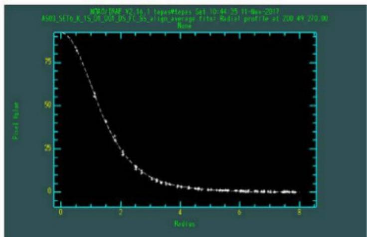
Figure 3.6: Top: TIRCAM2 instrument mounted with the side-port1 of the telescope. Bottom-left: The stellar image of a source observed with TIRCAM2 in the night of 16th Oct 2017. Bottom-right: The radial profile of the source is measured to be 0".45 FWHM.
