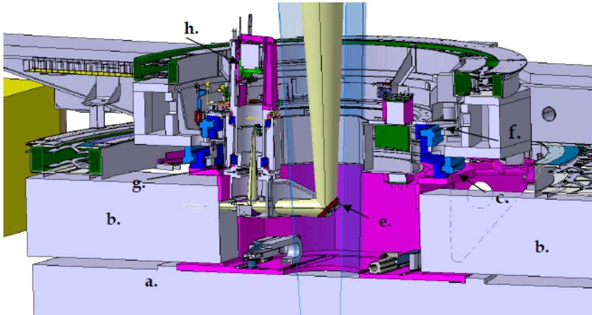
Figure 3.2: ARISS (Adapter rotator instrument interface structure) : a- main instrument envelope, b. side-port instrument envelope, c- rotator bearing, e- pick-off mirror, f- adaptor bearing, g-turn table, h- optical bench with guider camera and wavefront sensor.
