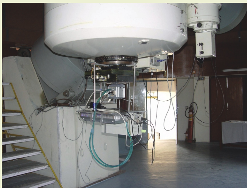
Figure 14. The new 512 X 512 frame transfer CCD recently installed for characterization at the back-end of the 104-cm Sampurnanand telescope of ARIES. This instrument will be one of the back-end instruments for the new upcoming 1.3-m telescope at Devasthal.
