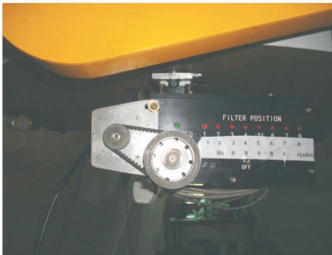
Figure 53. Automatic filter wheel assembly used in 130 cm telescope
