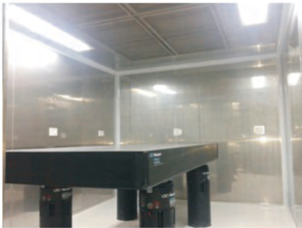
Figure 37. The class 10,000 clean room facility with vibration free table installed at optics lab, ARIES, Nainital.
