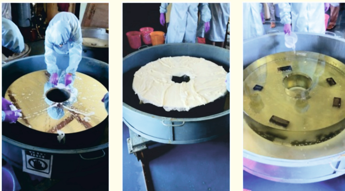
Figure 64. Cleaning M1 using soap solution (left), using KOH soaked cotton pads to remove old coating (centre) and rinsing with distilled water after coating removal (right).
