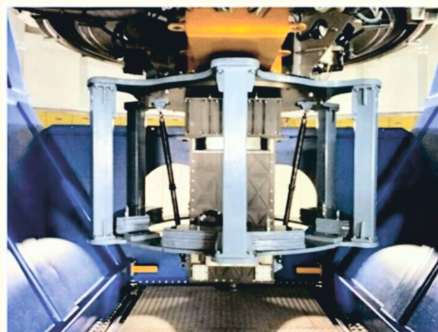
Figure 49. The FOSC-type instrument mounted at the Cassegrain focus of the 3.6m DOT for conducting various engineering tests. The anti-flexure units (black pipes) are mounted on the sides of the spectrograph to prevent mechanical flexure during the movement of the spectrograph.
