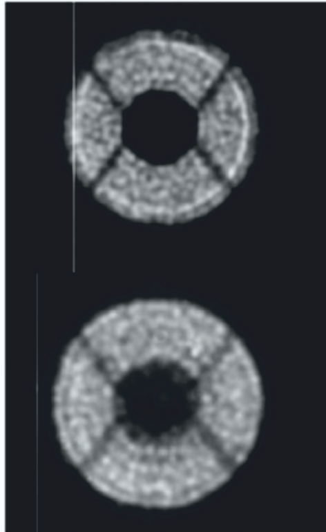
Figure 58. The in-focus and out-focus images were recorded using 4k CCD imager in night of 20 th March 2017. This indicates satisfactory alignment of primary and secondary mirrors of 3.6m DOT.
