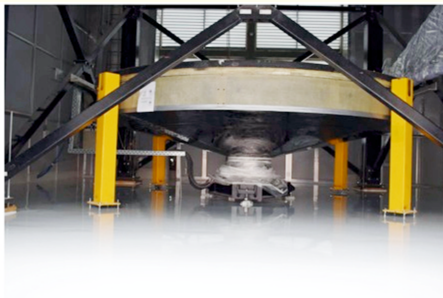
Figure 37. View of the ILMT mirror, the air bearing and four safety yellow pillows to prevent any switchover of the mercury bowl.
