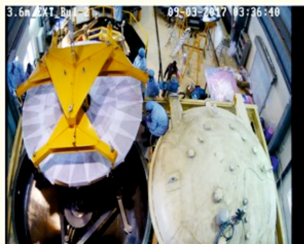
Figure 63. Removing old coating using KOH solution (left); placing mirror inside coating chamber using crane (right).
