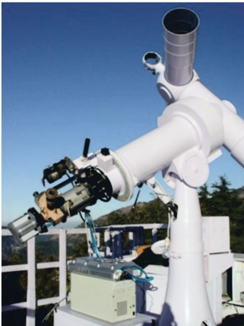
Figure 60. The 15cm Coudé solar tower telescope for solar observations.
