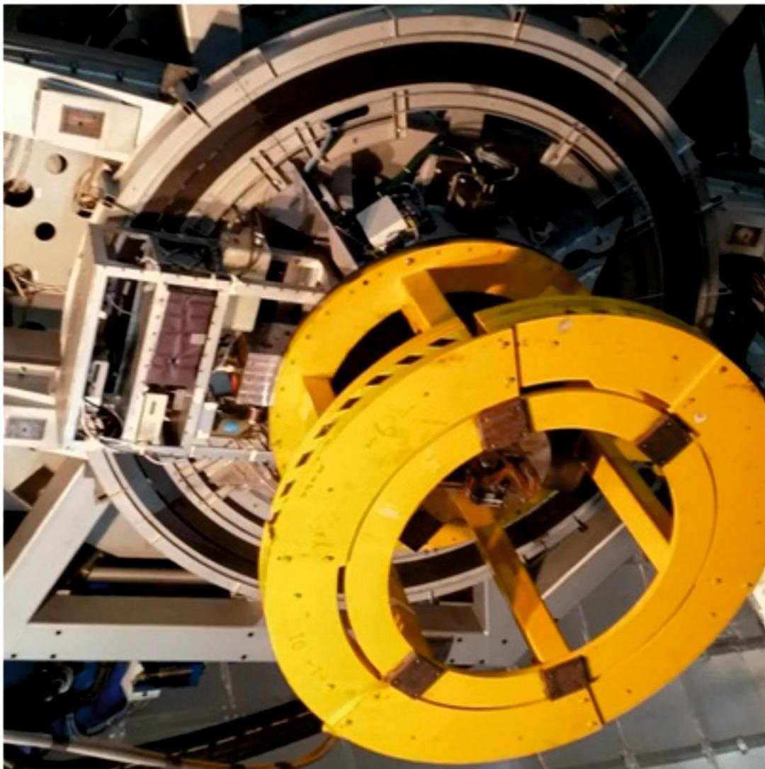
**Figure 44.** The TIRCAM2 instrument mounted at the sideport of 3.6m DOT. The yellow instrument structure is mounted on main axial port.
