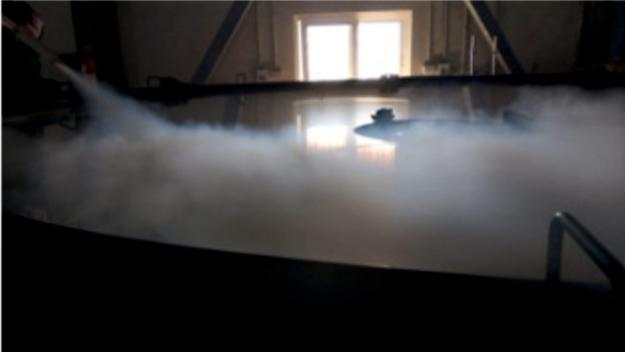
**Figure 56.** CO<sub>2</sub> cleaning of 3.6m DOT primary mirror.
