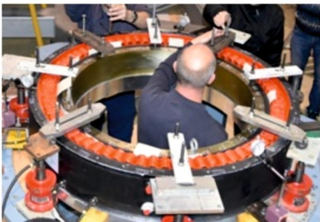
**Figure 64.** Tilt correction of stator.
