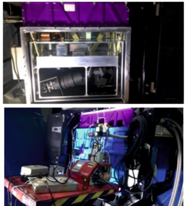
**Figure 58.** TANSPEC with Dewar opened condition (top), Evacuation of dewar after integrating with DOT.
