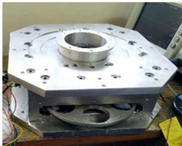
**Figure 67.** Polarimeter filter wheel assembly.
