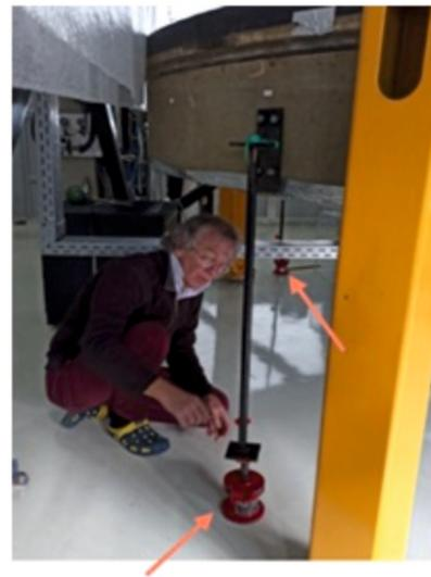
**Figure 36.** Four car-jacks (two of them are shown) used to lift the mirror to orient it properly with respect to the air-bearing.
