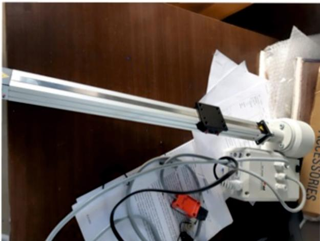
**Figure 38.** After assembling the linear stage with the hand-wheel and making electrical connections with the limit switch.
