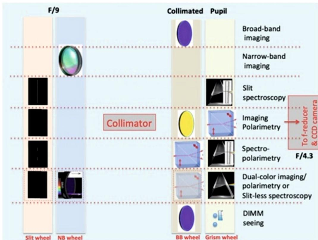
Figure 39. Various commissioned and planned observing modes on the AD-FOSC.
