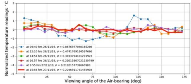
**Figure 35.** Temperature readings around the air-bearing at different times. The dashed plot represents the readings before the fans inside the insulating box were switched on. The thick continuous line represents the temperature readings after the air-bearing was supplied with clean air while the fans are still active.
