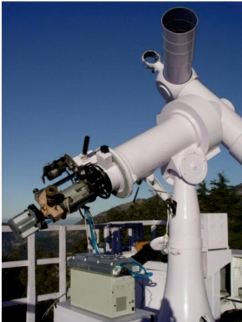
**Figure 52.** The 15cm Coude solar tower telescope for solar observations.
