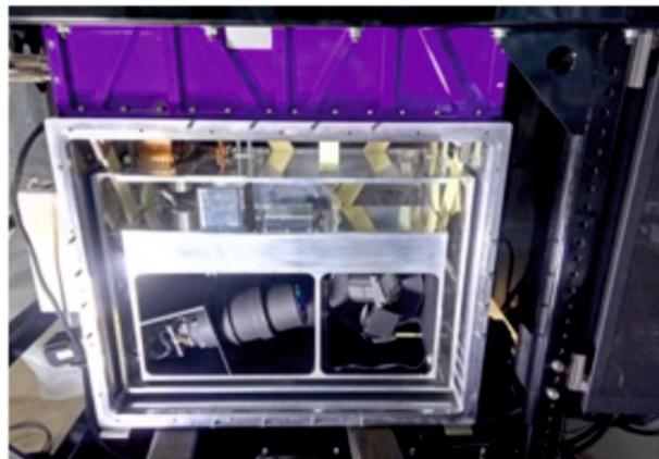
**Figure 68.** NSPEC Dewar opened for maintenance.
