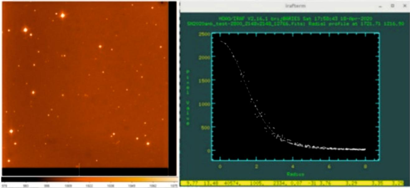
**Figure 50.** A 30s R-band image of a  $6.5 \times 6.5$  arcmin field centered at SLSN 2020ank using IMAGER with pixel binning of  $2 \times 2$  (left); Image profile of a stellar source of the same field. The PSF FWHM is 3.25 pixels (0.62 arcsec).
