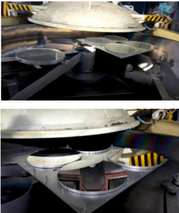
**Figure 57.** TACTIC mirrors coating set up, before coating (top), after coating (bottom).
