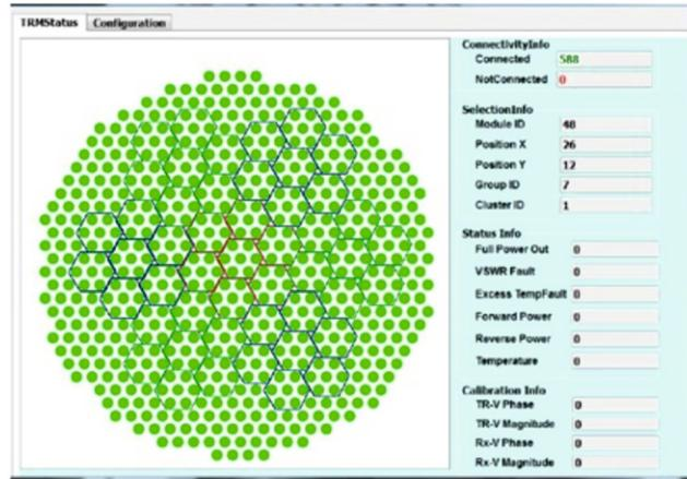
**Figure 33.** Readiness (green color) of all 12 clusters of ARIES ST Radar. One cluster consists of 49 TRMs and thereby making total 588 TRMs.
