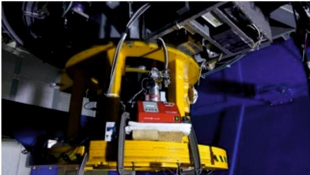
**Figure 59.** Evacuation TIRCAM2 which was integrated in the side port of 3.6m DOT.
