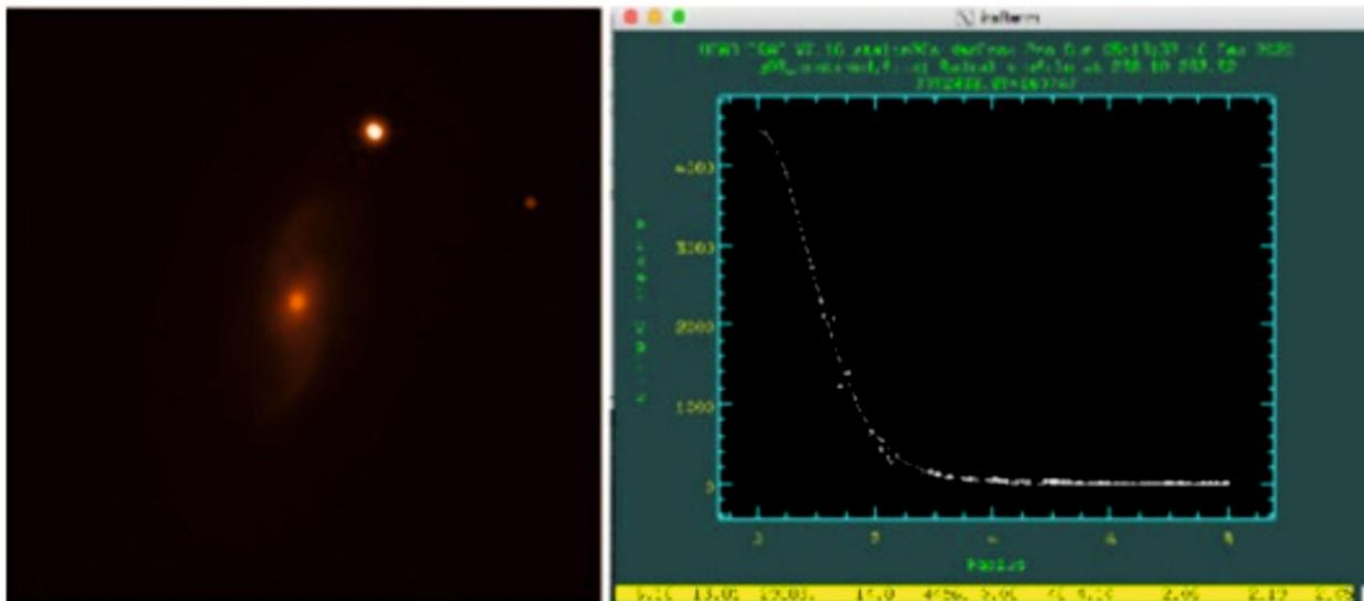
**Figure 49.**  $1 \times 1$  arcmin FOV J-band image centered on a galaxy with integrated exposure of 10 min observed with TANSPEC (left); radial profile of the stellar source in the image is measured to be 0.5 arcsec FWHM.
