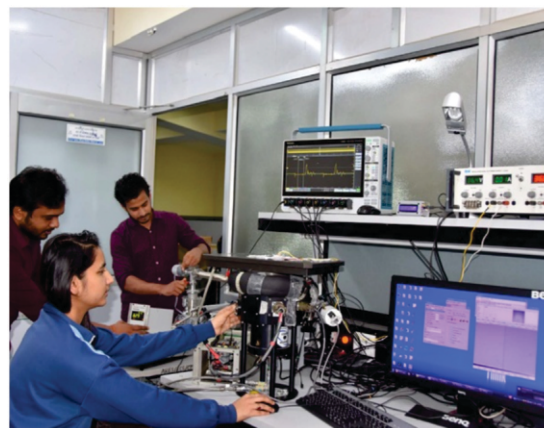
Figure 26. ARIES students utilizing the training area and interdisciplinary facilities in the laboratory for learning and characterizing a 4kx4k CCD camera.
