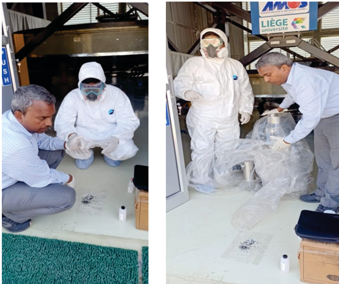
Figure 54. Left panel: Sprinkling sulphur impregnated charcoal around the contaminated area. Right panel: Using a mercury vacuum cleaner to clean the contaminated area.
