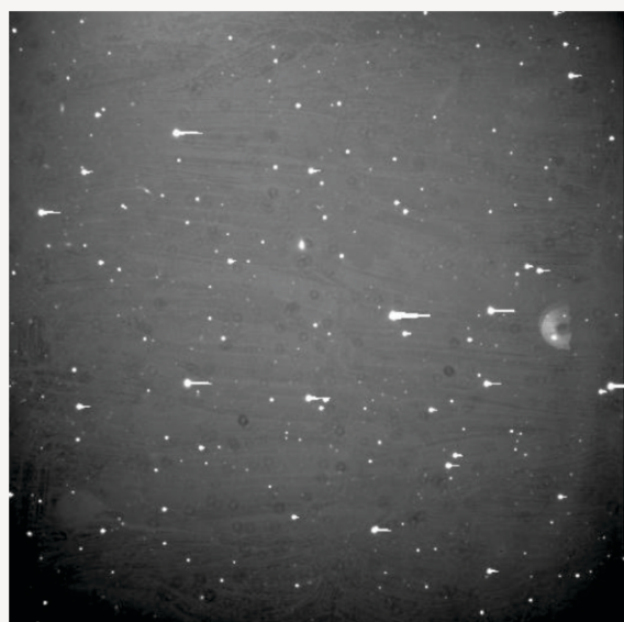
Figure 58. Left: A 15-min r-band image recorded with ADFOSC, without the telescope guider, on 14 March, 2022. The FOV is 13' \times 13' . Right: The PSF FWHM of the stellar profile was measured to be around 3.6 pixels, i.e. 1.4 arcsec.
