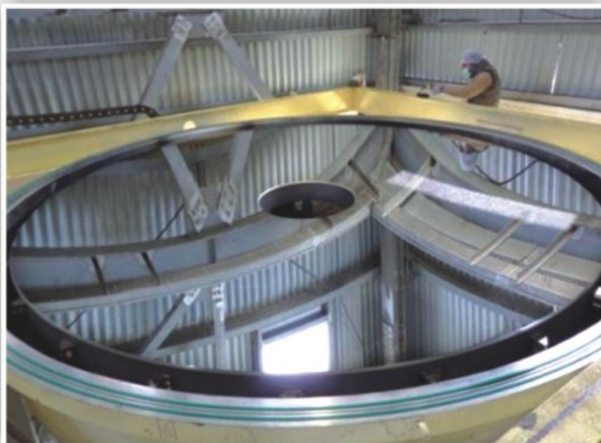
Figure 40 : The picture of freshly coated 3.7m diameter primary mirror of 3.6m devasthal optical telescope.
