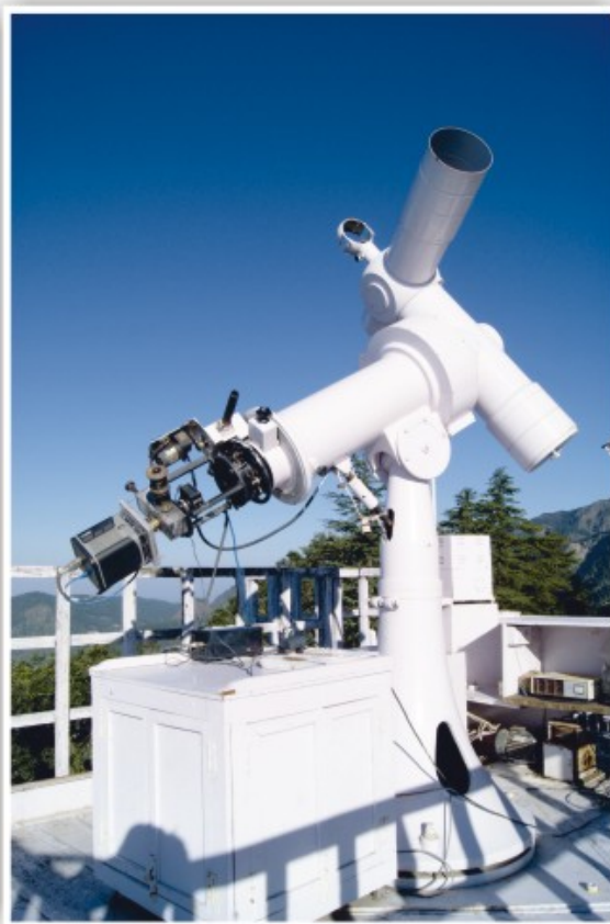
Figure 73. 15-cm Coude Solar tower telescope for solar observations.
