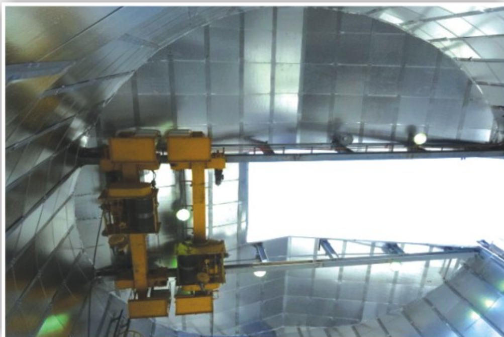
Figure 37 : Both the under-slung cranes of 10T capacity are seen in yellow. These are installed in the dome of 3.6m telescope enclosure building.
