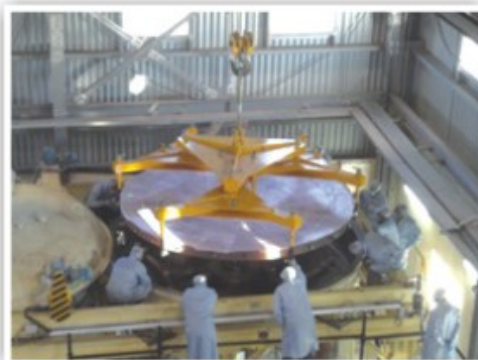
Figure 84. cleaning of the primary mirror (top), placing the mirror inside the coating chamber (bottom).
