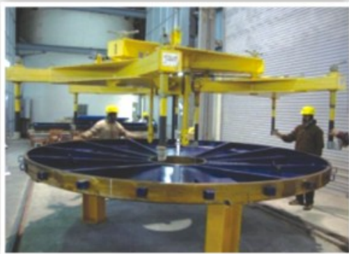
Figure 47. Rehearsals for lifting the mirror using the handling tool are being carried out using the dummy mirror.
