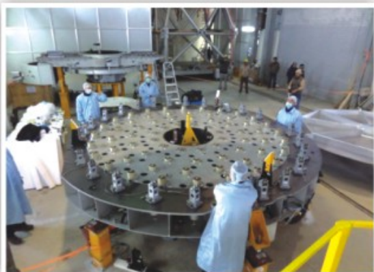
Figure 55. Balancing of the mirror cell is in progress. This was carried out by the AMOS.
