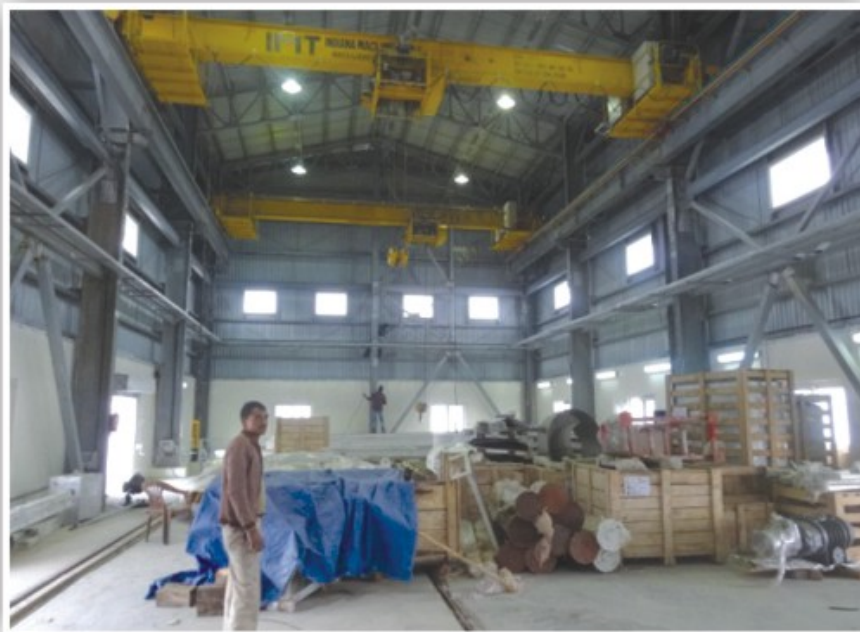
Figure 38 : Both the single-girder cranes of 10T capacity each are seen in yellow. These are installed in the extension building of 3.6m telescope enclosure.
