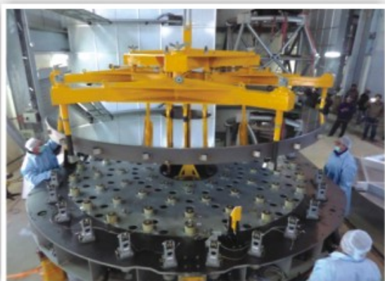
Figure 56. The mirror is being lowered onto the M1 cell.
