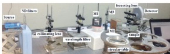
Figure 81. Experimental set up of VW method for reflectivity measurements of coated sample.
