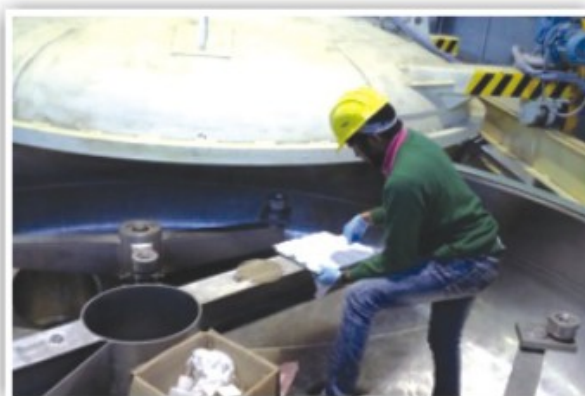
Figure 46. Loading of the sample glass on the sample holder for coating.
