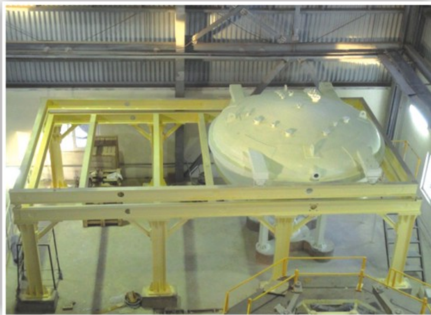
Figure 39 : The as-built picture of 3.7m diameter Aluminium coating plant at Devasthal. This facility has been installed in the extension building of 3.6m telescope enclosure. A portion of mirror washing unit is also seen in the foreground.
