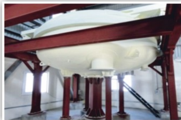
Figure 43. The coating chamber just after it got installed in the extension building and before the pumps and other gadgets were attached to it.
