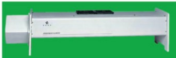
Figure 75. Photograph of three wavelength Integrating Nephelometer operational at ARIES.
