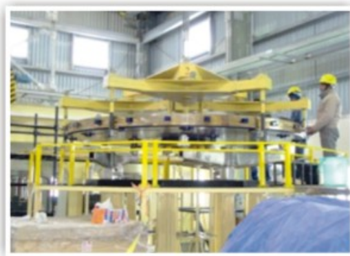
Figure 48. The mirror washing unit is getting examined using the dummy mirror.
