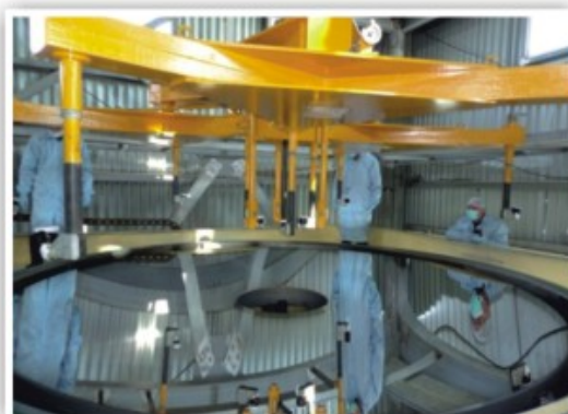
Figure 53. The mirror is getting lifted using the mirror handling tool.
