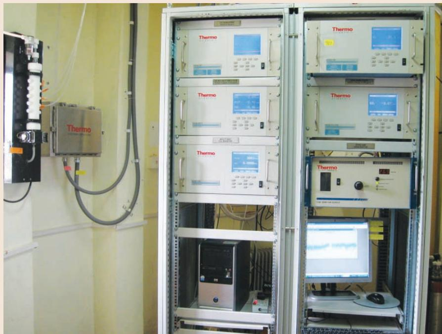
**Figure 24.** Different analyzer for O<sub>3</sub>, CO, NO, NO<sub>y</sub>, SO<sub>2</sub> at ARIES.
