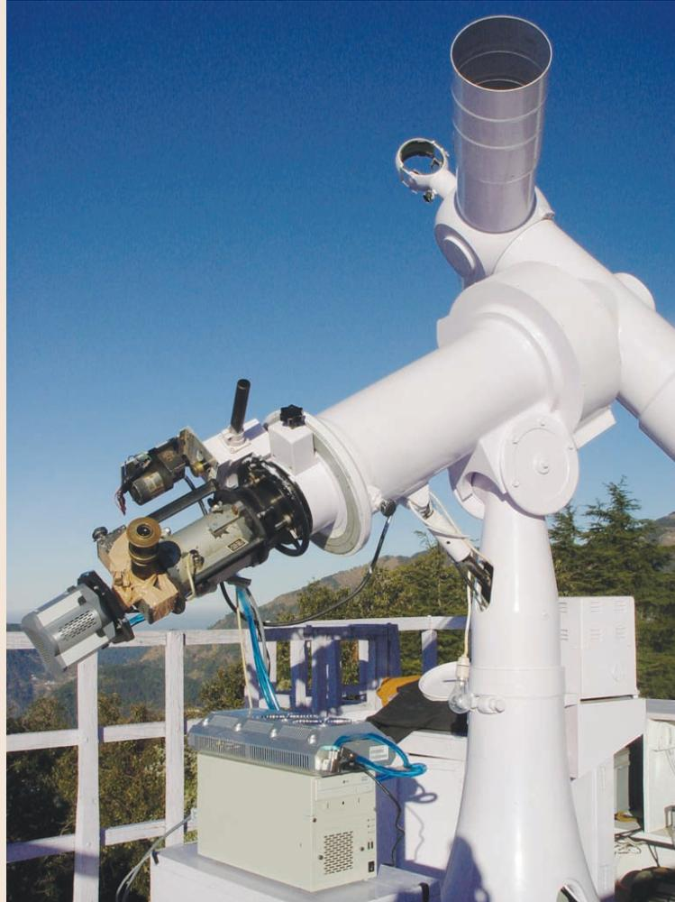
**Figure 23.** 15-cm Coude Solar Tower Telescope for solar observations.
