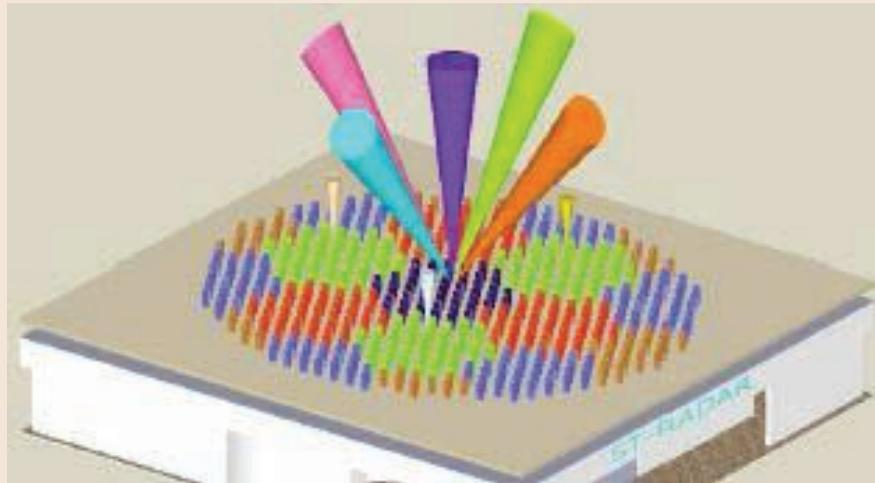
**Figure 30.** Schematic diagram of upcoming ST Radar, with display of antenna array in a circular aperture, at ARIES, Nainital.
