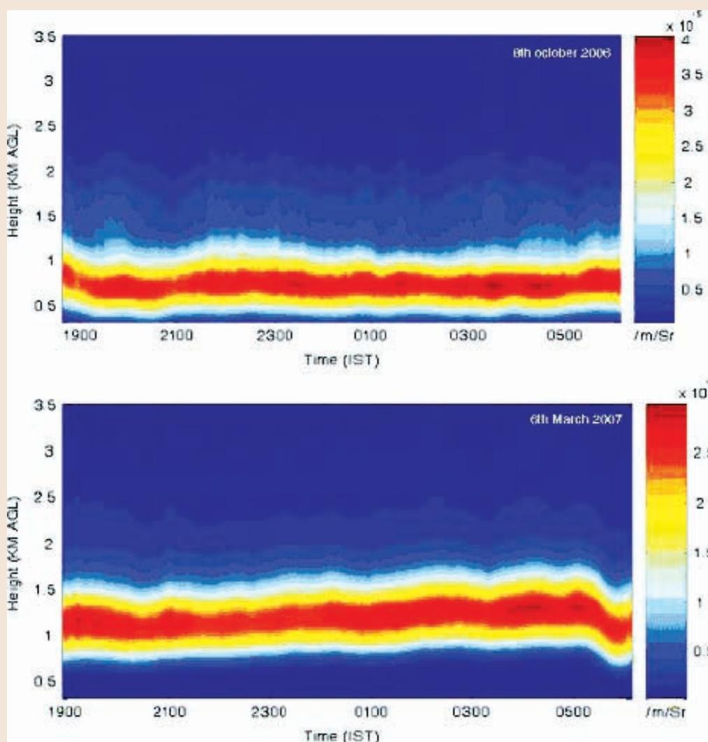
**Figure 20.** Night-time variation of the attenuated backscatter return, beta (1/m/sr) observed on 8 October 2006 (upper panel) and 6 March 2007 (lower panel).
