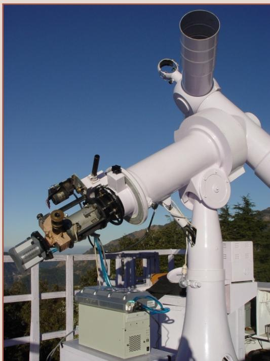
**Figure 22.** 15-cm Coude Solar Tower Telescope for solar observations.
