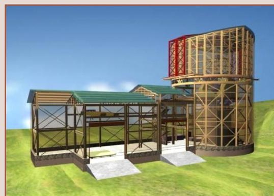
**Figure 25.** The concept design of the 3.6-m Devasthal Optical Telescope.
