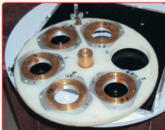
**Figure 28.** Filter disc of backend instrument interface for 1.3-m telescope.
