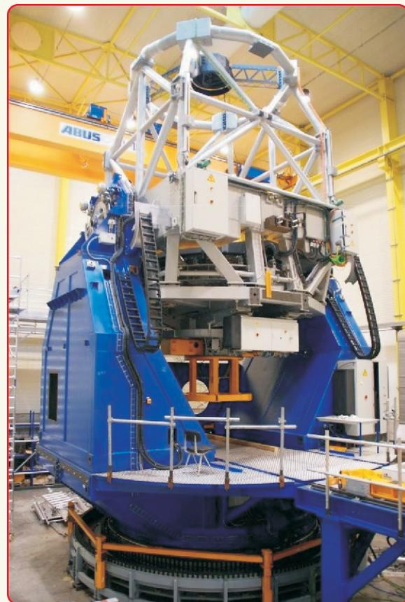
**Figure 30.** Fully assembled 3.6-m telescope with dummy mirrors at AMOS workshop.
