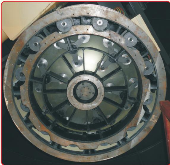
**Figure 29.** View from bottom of primary mirror cell of Schmidt telescope containing primary mirror floating on axial and radial supports.
