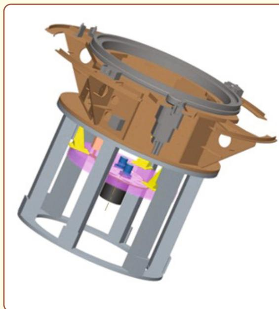
**Figure 3.** The mounting plan for the 4kx4k optical imager with the instrument interface of the 3.6m DOT.
