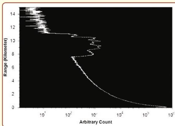
Contour plot of range corrected signal (top panel) and typical altitude profile of photon count (bottom panel) for 23 November 2011.
