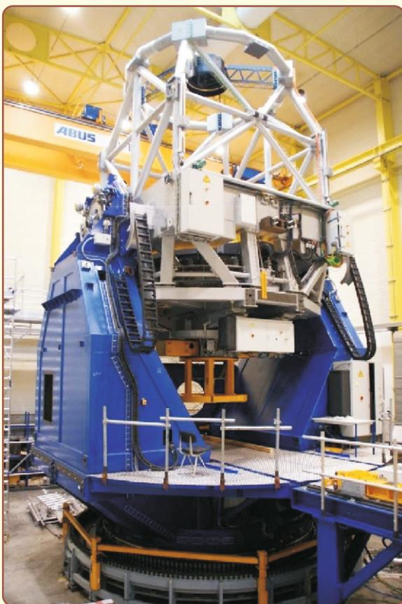
**Figure 1.** Fully assembled telescope with real mirrors at AMOS workshop. The Dummy instrument with one axial port and two side ports are shown in yellow.
