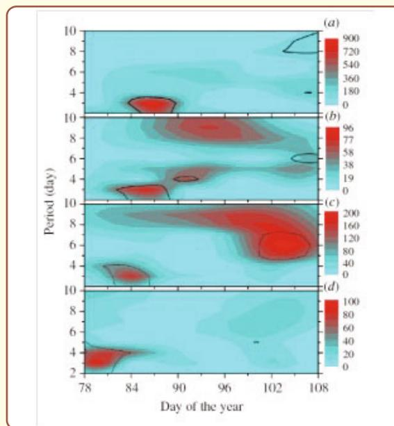
**Figure 2.** (a) Temperature variability plot of LiDAR (red) and MLS (black) during the March to April 2007 period for: (a) 80 km, (b) 70 km, (c) 60 km and (d) 50 km over Gadanki. (b) Wavelet power spectra of LiDAR temperature over Gadanki with respect to day of the year (DY) and period for: (a) 80 km, (b) 70 km, (c) 60 km and (d) 50 km. The solid lines represent the 90% significance level.
