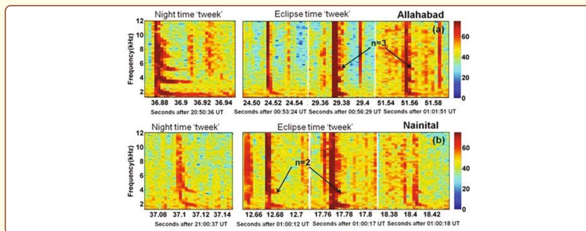
The tweek examples observed at (a) Allahabad and (b) Nainital stations on 22 July 2009 before, during and after the eclipse totality. The second and third harmonic tweeks are indicated as  $n = 2$  and  $n = 3$ . On the left sides of Figures 2a and 2b, tweeks observed in the nighttime on 22 July 2009 are shown.
