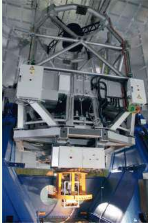
Figure 43. The TIRCAM2 mounted at the axial port of the 3.6m DOT.
