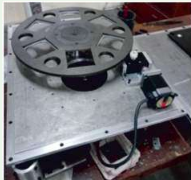
Figure 61. Filter wheel unit.
