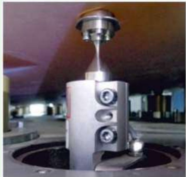
Figure 53. Shim of thickness 1100 micron placed at axial definer 3.
