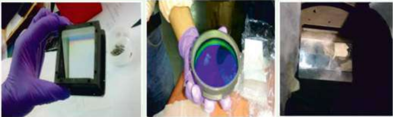
Figure 57. Grism (left), filter (center) and slit (right) in their respective mechanical holders
