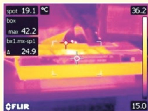
Figure 25. Testing of in-house developed TRM in RF laboratory at ARIES. Thermal dissipation testing is also done.
