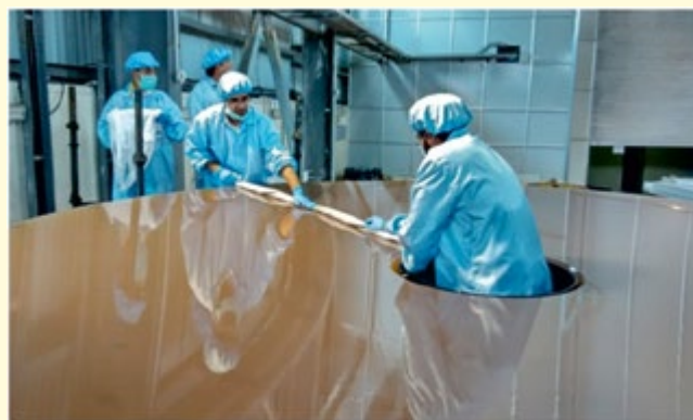
Figure 55. Drying the mirror surface using lint free towels.
