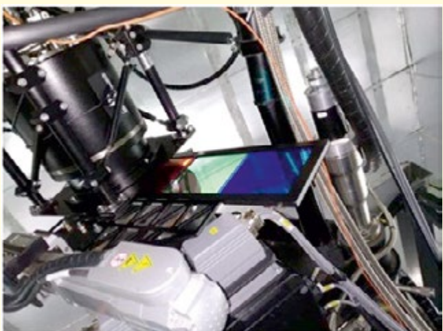
Figure 29. Installation of the tray with the SDSS broadband filters on the Socabelec mechanical interface at the prime focus.
