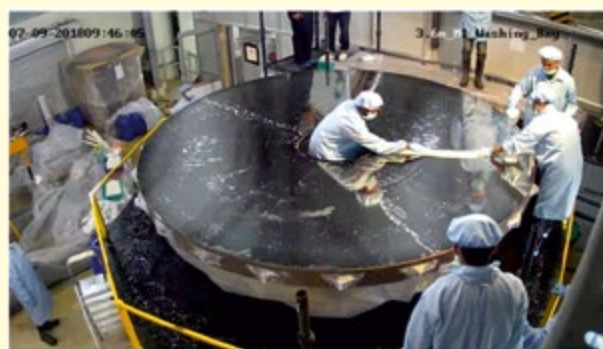
Figure 53. Cleaning the mirror using cotton pads and soap solution.
