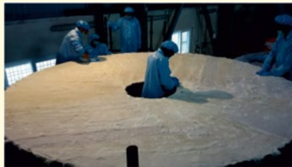
Figure 52. Covered the mirror surface with wet cotton pads and soap solution.
