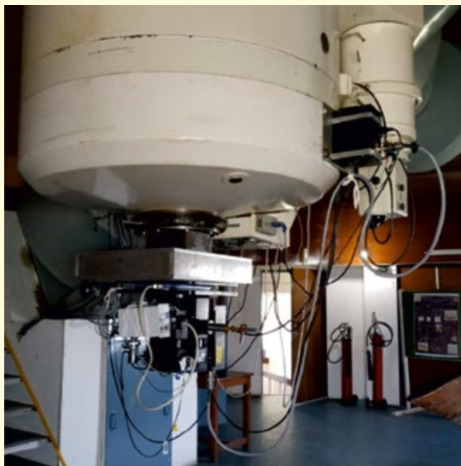
Figure 64. The whole setup installed with new 4kx4k CCD at 1.04m ST.
