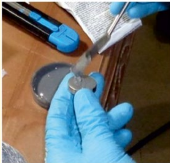
Figure 59. Applying glue to axial pad.
