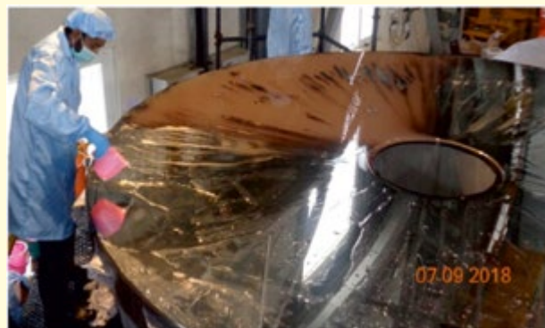
Figure 54. Pouring KOH solution to remove the old aluminium coating
