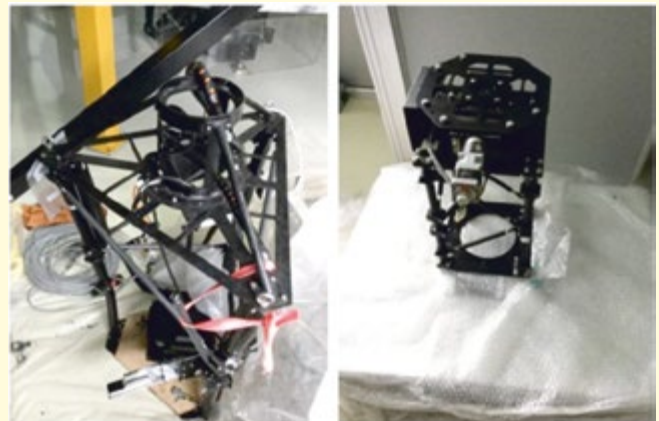
Figure 27. The mechanical interface (at left) and the interface's component to hold the CCD camera (at right).
