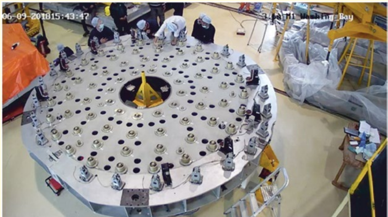
Figure 58. Inspection of mirror cell (actuators, radial supports etc.) after disintegrating primary mirror.
