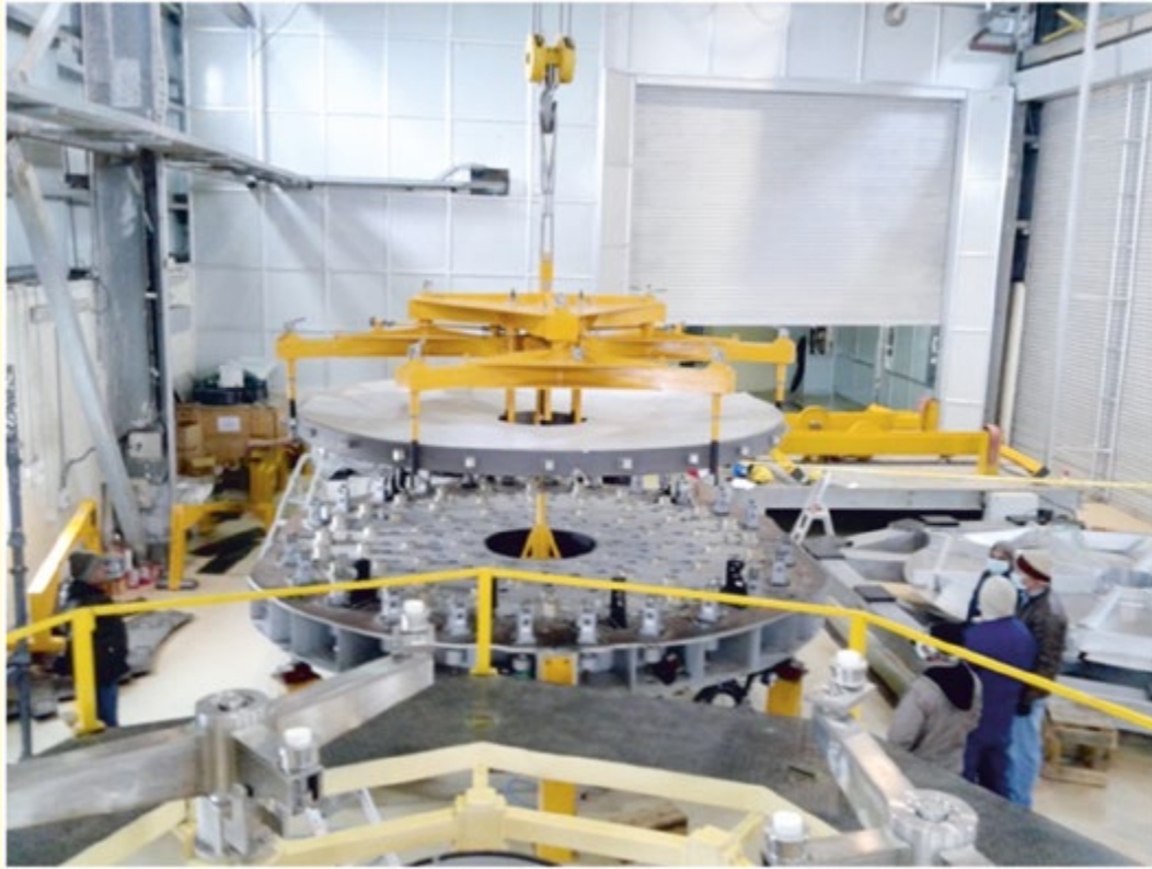
Figure 57. Lifting 3.6m mirror from mirror cell using mirror integration tool (yellow) and extension building crane.
