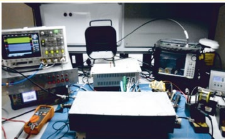
Figure 25. Testing of in-house developed TRM in RF laboratory at ARIES. Thermal dissipation testing is also done.
