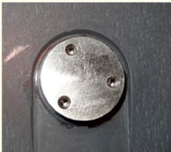
Figure 60. Axial pad after gluing to mirror surface.
