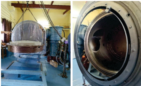
Figure 89. Left: Primary mirror of 104cm ST ready to be loaded inside the coating chamber, Right: The primary mirror after fresh aluminium coating.
