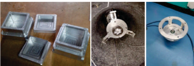
Figure 84. Mechanical mounts fabricated in the mechanical workshop.
