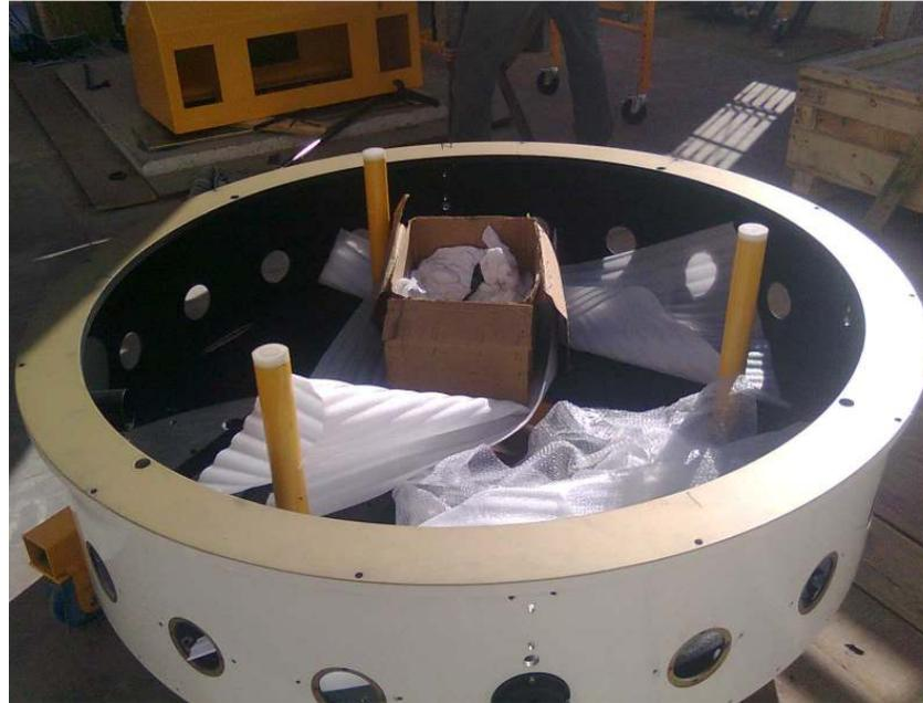
Figure 1: mirror cell placed on the mirror inserting trolley
