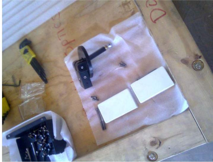
Figure 2: Radial support having a radial rod and counter weights
