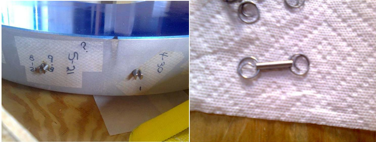
Figure 6: radial rods fixed in the invar blocks (left) clevis pins to fix the rods in invar blocks (right)
