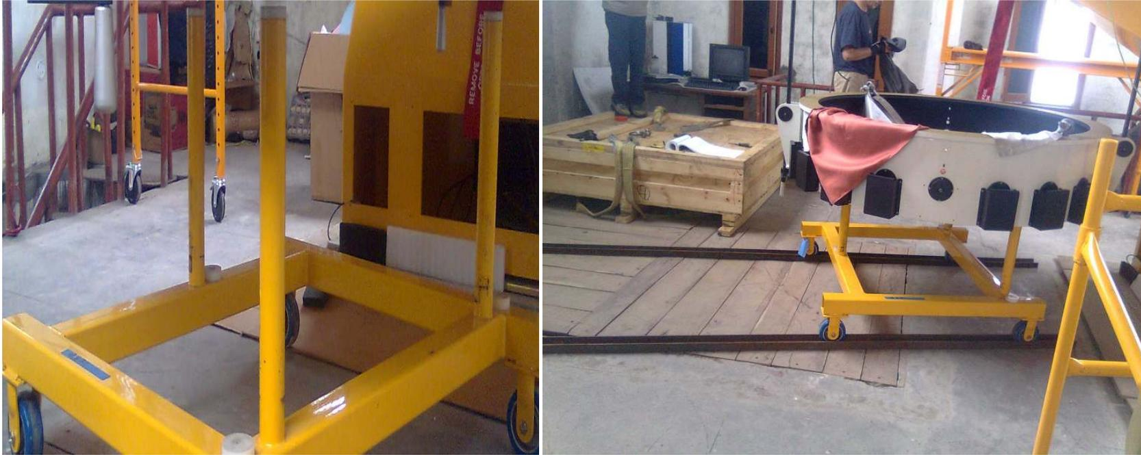
Figure 12: mirror cell inserting trolley (left) guiding rails (right)
