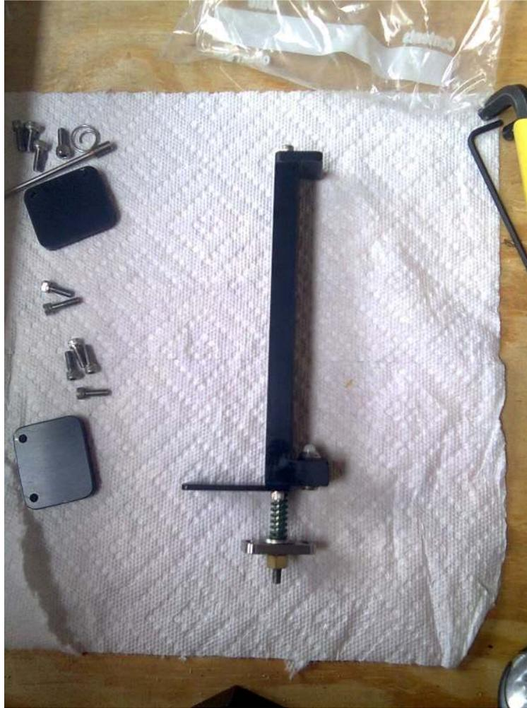
Figure 10: axial defining supports (a bracket assembly plunger and spring at the end of the rod)
