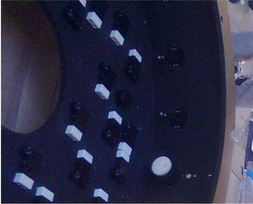
Figure7: axial (back) supports at the base of the mirror (left) map of the axial back supports (right)
