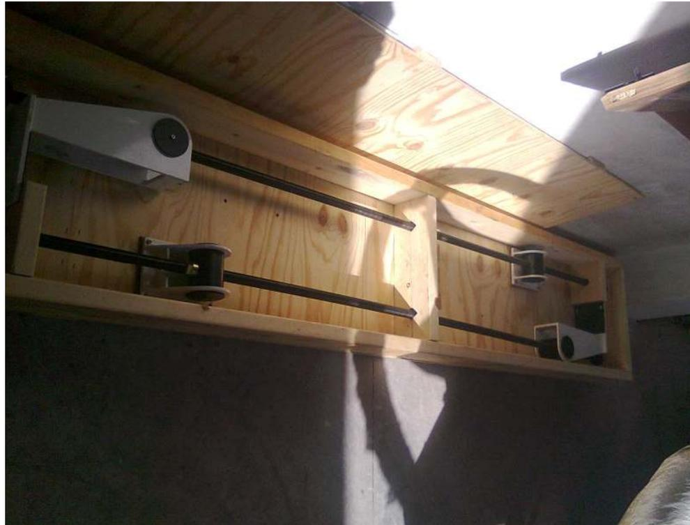
Figure11 : MCLA tool for lifting the mirror cell.
